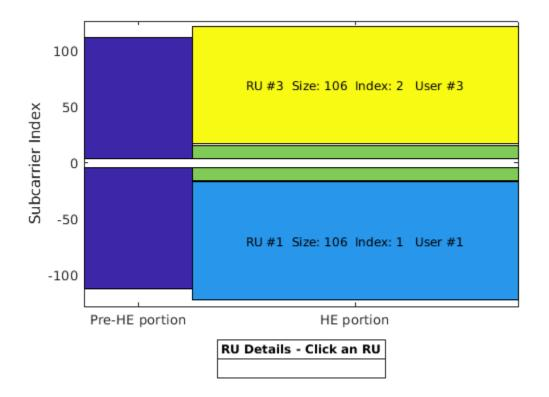
The ruInfo method provides details of the RUs in the configuration. In this case we can see three users and three RUs.
