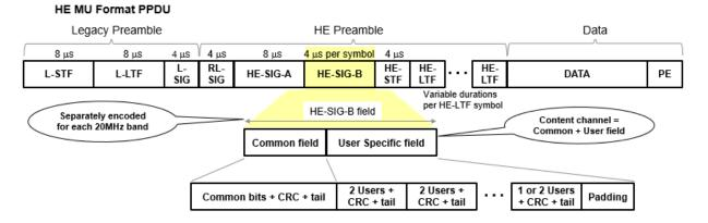
The format of the common field is defined in Table 28-23 of [1]. The RU Allocation subfield in the common field of HE-SIG-B consists of 8 bits that indicate this information for each 20 MHz PPDU bandwidth.
