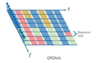
The values specified in the AllocationIndex property correspond to the 8-bit indices for each 20 MHz subchannel in the first column of Table 28-24 in [1]. The allocation indices define the number of RUs, RU sizes, and number of users assigned to each RU. When SIGB compression is enabled, the number of users is determined by decoding the HE-SIG-A field. When SIGB compression is disabled, the number of users is determined by decoding the HE-SIG-B common field.
